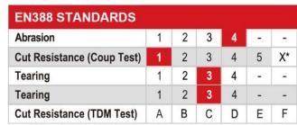
\*If the coupe test provides a 3 or above it is marked as an "X" for not applicable and uses the TDM 100 test instead
